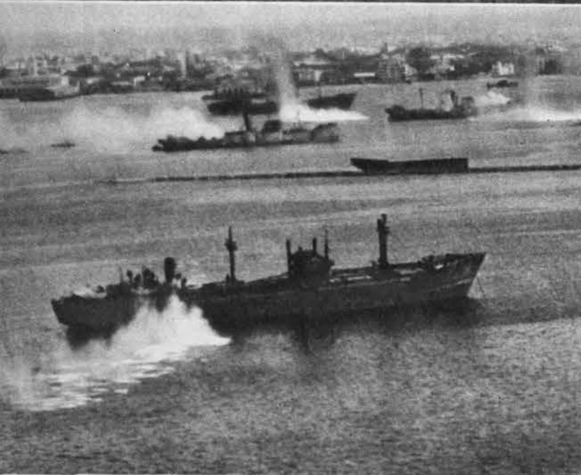
Triangular bow, chopped-off stern mark Sugar Baker Love as an "economy" hull design. Sturdy masts, booms and big hatches indicate it is a large cargo vessel. Note four kingposts built into bridge.
